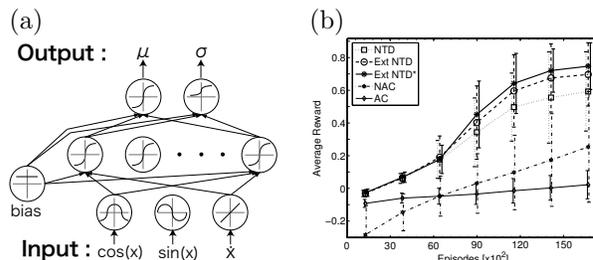
Figure 3: Swing-up pendulum problem; (a) The policy is a three-layer neural network with 10 hidden units. (b) The average rewards over 30 independent runs. Comparison among PGs under the improper RBF setup,  $[5 \times 5]$ , for the state value estimation. Extended NTD\* is the alternative algorithm computing  $b_1$  analytically.
